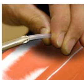
2.5-From the inside of the kayak, pass the trimmed section inside the brass fitting. From the outside, pull on the tubing until the trimmed section is completely out of the boat. Cut the trimmed section, heat the end of the tubing with a lighter and use a star screwdriver to widen the opening. From the inside of the kayak, pull on the tubing to bring the widened section as close as possible to the brass fitting;
