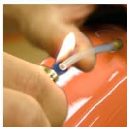
2.5-From the inside of the kayak, pass the trimmed section inside the brass fitting. From the outside, pull on the tubing until the trimmed section is completely out of the boat. Cut the trimmed section, heat the end of the tubing with a lighter and use a star screwdriver to widen the opening. From the inside of the kayak, pull on the tubing to bring the widened section as close as possible to the brass fitting;
