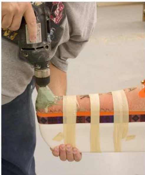
1-Rudder Installation: drill a hole with a 3/8 bit on the kayak stern.
