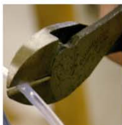
2.5-From the inside of the kayak, pass the trimmed section inside the brass fitting. From the outside, pull on the tubing until the trimmed section is completely out of the boat. Cut the trimmed section, heat the end of the tubing with a lighter and use a star screwdriver to widen the opening. From the inside of the kayak, pull on the tubing to bring the widened section as close as possible to the brass fitting;
