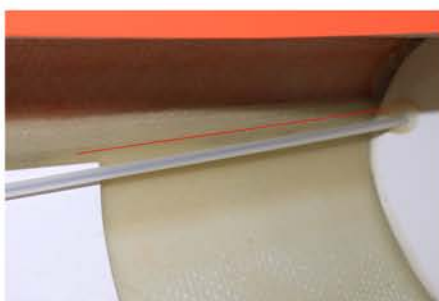
2.2-Drill 2 holes in the bulkhead with a 1/8 bit and refer to the seat to adjust the height of the holes;
