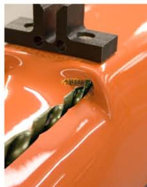
2- Drill 2 well-centered holes with a 13/64 bit (on the stern). Make threads with a 1/4-20 screwing die (optional);
