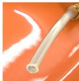
2.5-From the inside of the kayak, pass the trimmed section inside the brass fitting. From the outside, pull on the tubing until the trimmed section is completely out of the boat. Cut the trimmed section, heat the end of the tubing with a lighter and use a star screwdriver to widen the opening. From the inside of the kayak, pull on the tubing to bring the widened section as close as possible to the brass fitting;
